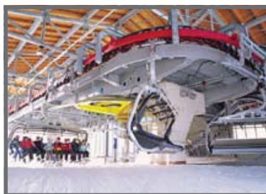
Guide rails fixings
