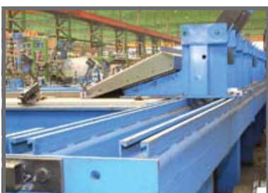
Welding jig-locomotive construction
