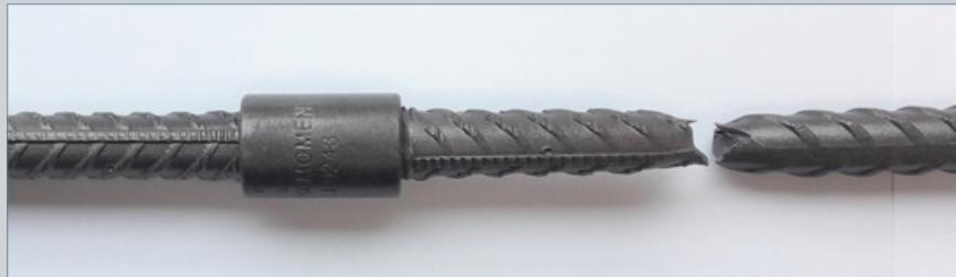
Moment JoinTec Type A Couplers have been tested to satisfy the requirements of CARES Appendix TA1-F for Couplers with reinforcing bars to BS4449 Grade B500B as appropriate. The testing comprised the following elements:
