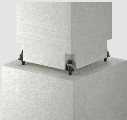
Figure 4: Tighten upper and lower nuts using suitable wrench
