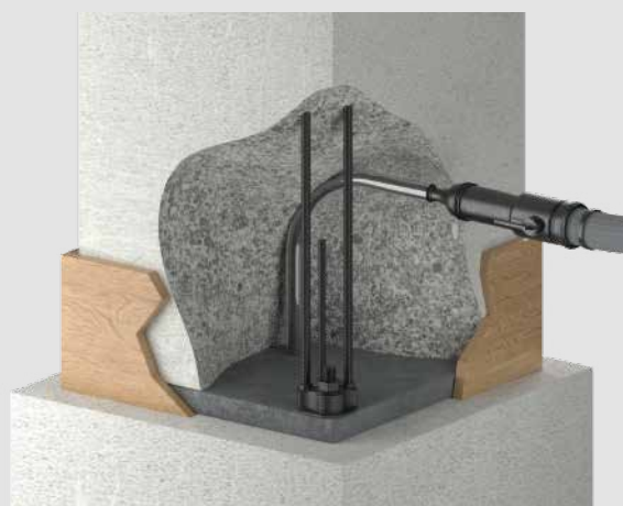
Figure 6: Grouting process from cast-in pour-pipe
