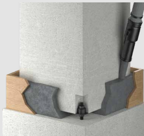
Figure 5: Grouting process from side
