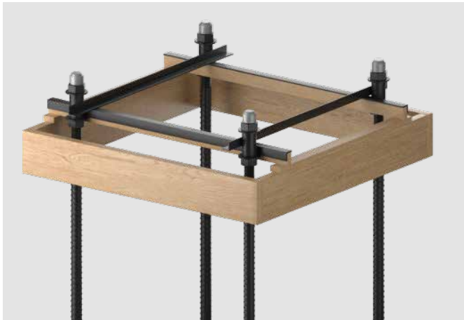
Figure 2: Assembly of positioning bolt and recess formers
