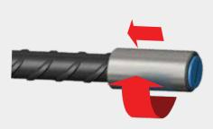
Screw the coupler to the rear of the thread on the fixed bar and lock tight. The bar end should be central within the coupler.
