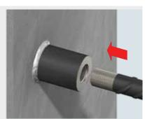
When ready to extend, position the continuation bar into the sleeve.
