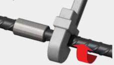
3 Tighten the joint using a wrench on the continuation bar. After tightening there should be no more than 4mm of exposed thread; for size 20mm and below, or 6mm for sizes 25mm and above.
