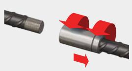
1 Screw the locknut followed by the coupler to the rear of the thread on the continuation bar.
