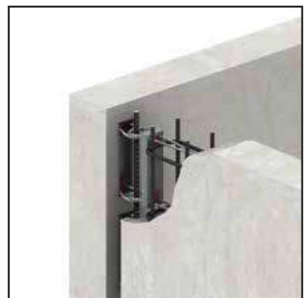
Conner Wall Connection
