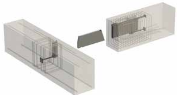
BSF Telescopic Beam Connectors – Designed for invisibly supporting beams off columns
