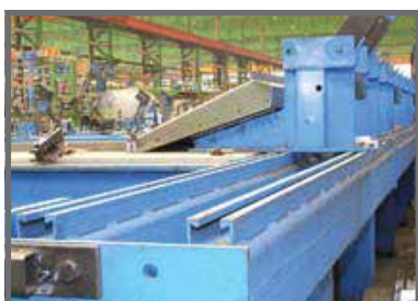
Welding jig-locomotive construction
