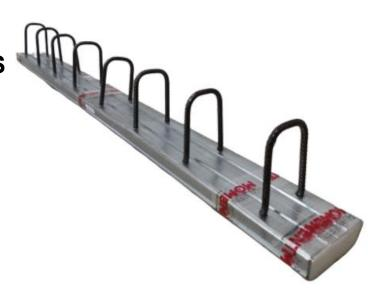
Check that the chosen dimensions of the Moment Bar Box correspond with the required concrete cover of the second concreting phase. Ensure that the End Cap (PE Foam) are in place at both ends of casing.
