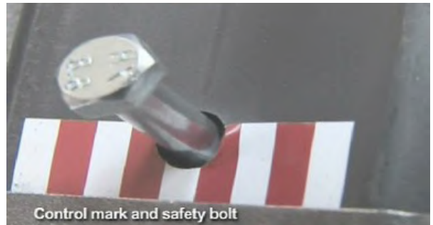
M12: Place the safety bolt in the hole
